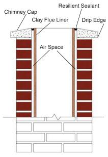
All masonry chimneys must be terminated with a cap that is 2 inches thick (minimum), extending 1½ inches away from the chimney wall with a drip edge. All caps must be center reinforced with ½ inch (min) galvanized hardware cloth. The top slope of the cap should be 10 degrees away from the flue liner. This cap may be cast-in-place or pre-cast concrete.
